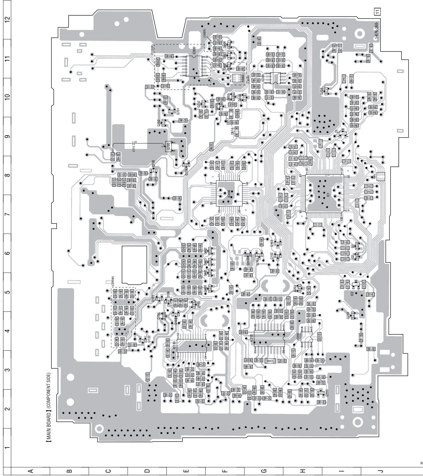
5-2. PRINTED WIRING BOARD – MAIN Board (Component Side) –
